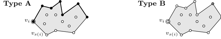
Fig. 4. The two types of pointgons we encounter in the purely triangle-based algorithm. A black point indicates a vertex belonging to V_p , a white point a vertex belonging to V_h , a grey point a vertex either in V_p or in V_h . The encircled point is the anchor. Thick lines indicate pieces of the perimeter of the input pointgon.
